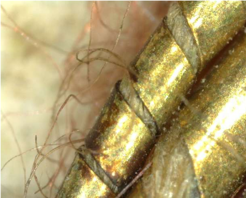
Fig.20 – Antao et al (2020) Henry VI Lincoln Charter, 1456 : metallic thread corrosion x120 magnification (dinoeye).1 [digital microscopy image] personal collection
