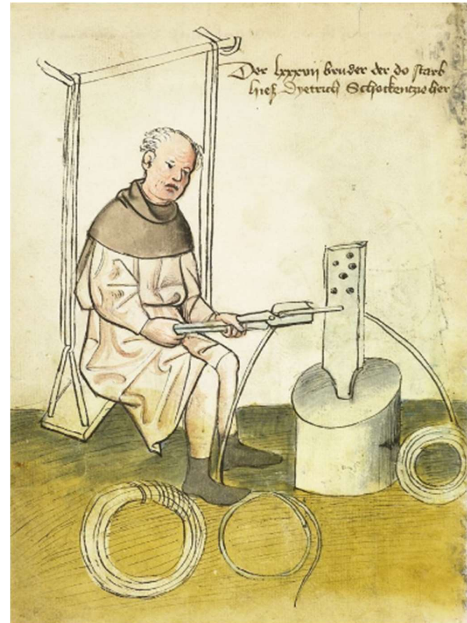
Fig.17 - Germanisches Nationalmuseum, 2020, Polbach Hausbach (MS 3227a) , 1389 : detail of use of wire draw plate [altered digital scan], Digitale Bibliothek
