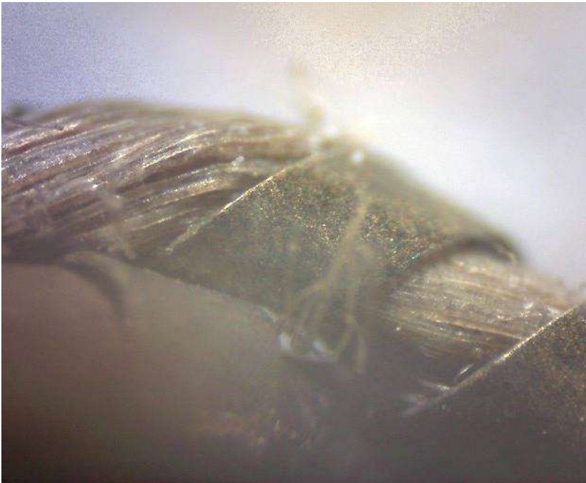
Fig.15 – Beirne (2020) Henry VI Lincoln Charter, 1456 : metallic thread x120 magnification.1 [digital microscopy image] personal collection
